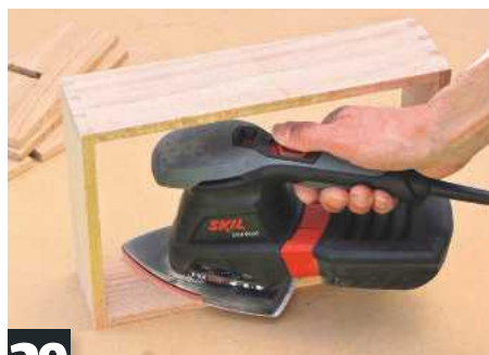
29 Rout small decorative chamfer along edges of tray and dividers. Sand with 180grit abrasive
